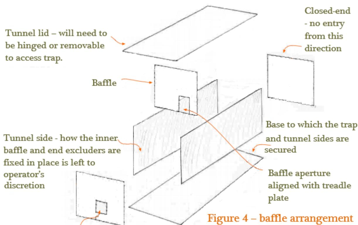
Figure 4 – baffle arrangement
